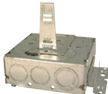
"UBS" Support Universal Back Side support to provide bracing on back of box for wall cavities 2-1/2" - 6" thick.
