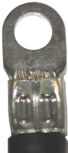
Close up of “M” Profile Crimp
