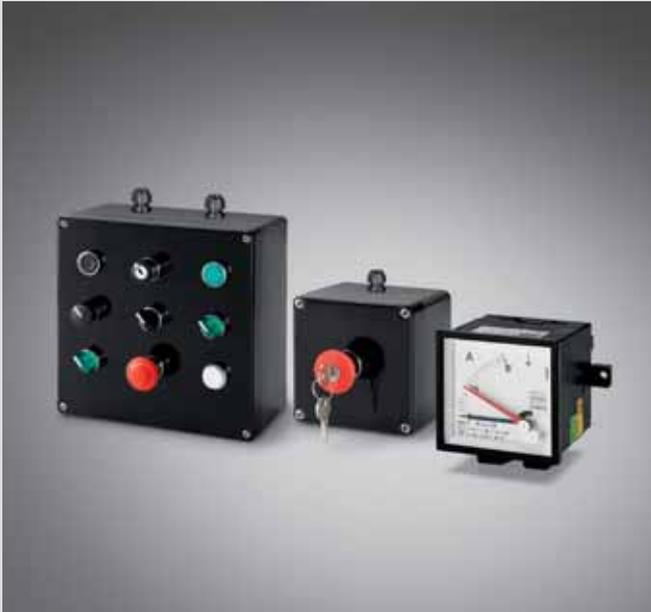
The ZENITH-P Series can be customised as a control station. The control stations can be assembled to house a broad range of actuators and components with separate ATEX-IECEX certification, including buttons, indicators, selectors, analogue instruments, etc. It is also possible to customise units including MCB, MCBO, RCD, transformers, disconnectors, fuses, timer or thermal relays, all with "Ex db eb" certification. They are available in preconfigured versions.
